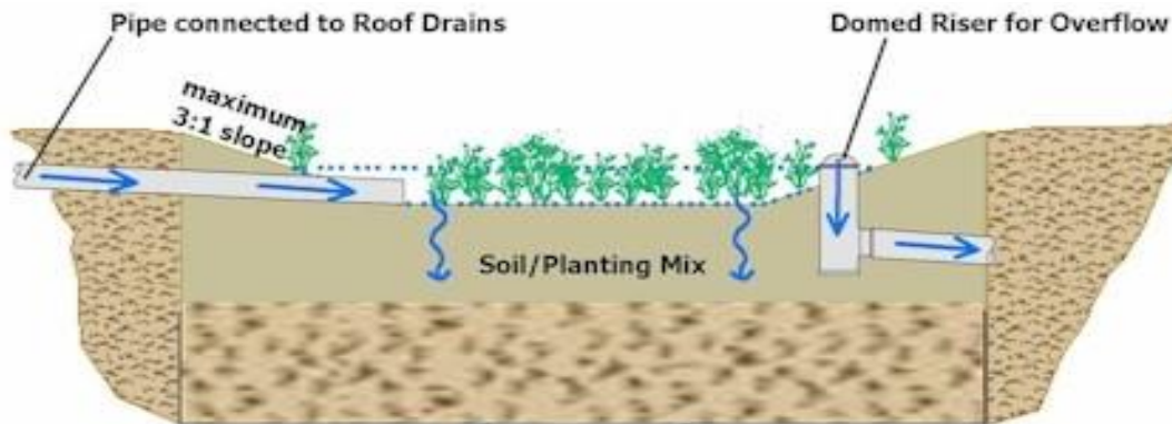
Figure 4: Cross-Section of Typical Rain Garden/Bioretention Area
